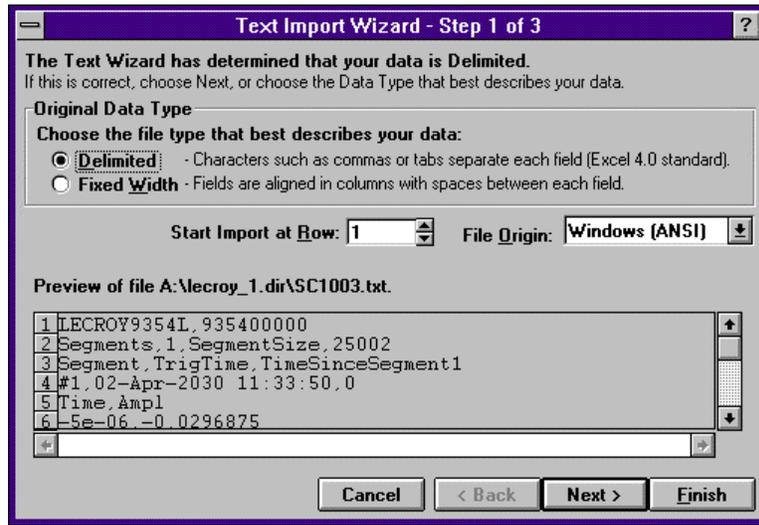
The next step allows the specific delimiter to be specified. The Spreadsheet format generated by the scope uses a comma (,) to delimit columns. Ensure that this is selected.
