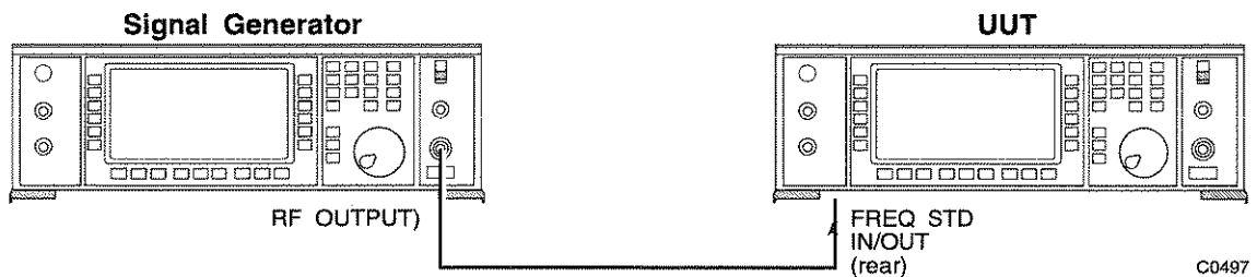
Fig. A-24 Frequency standard locking test set-up.
