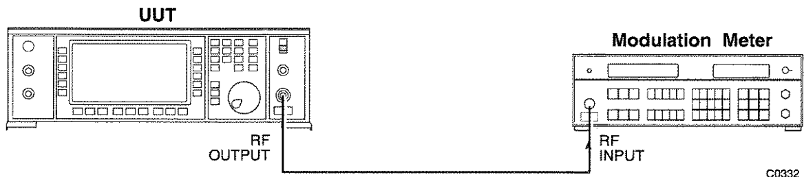
Fig. 5-1-9 Internal AM depth and distortion test set-up
