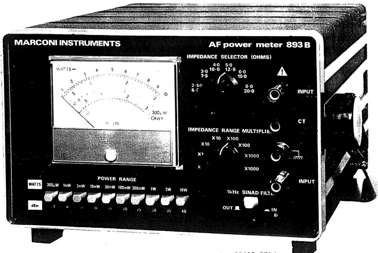
Fig. 1 AF power meter 893B (version 50893-321J with SINAD FILTER switch)
