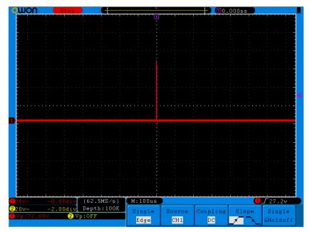
Fig.6-3 Capturing a Single Signal
