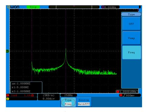
Fig.5-62 wave of Freq cursor measurement
