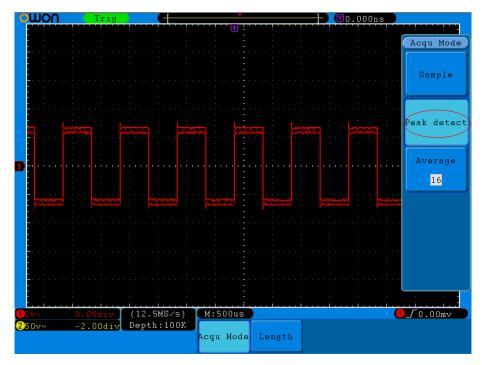
Fig.6-4 Signal with Noises
