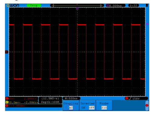
Fig. 5-2 AC Coupling Oscillogram
