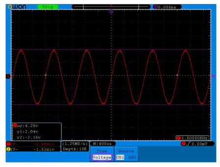
Fig.5-58 Waveform of Voltage Cursor Measurement
