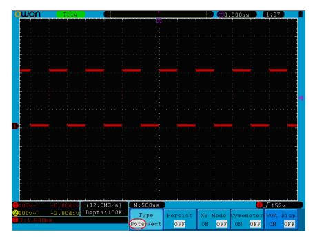
Fig.5-31 Display in Dots form
