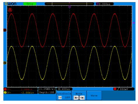
Fig.5-64 Autoscale Horizontal-Vertical multi-period waveforms
