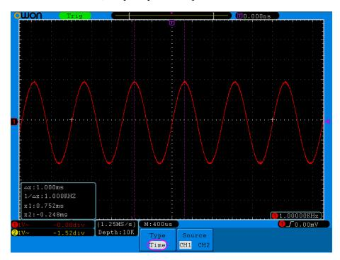
Fig.5-59 Waveform of Cursor Measurement
