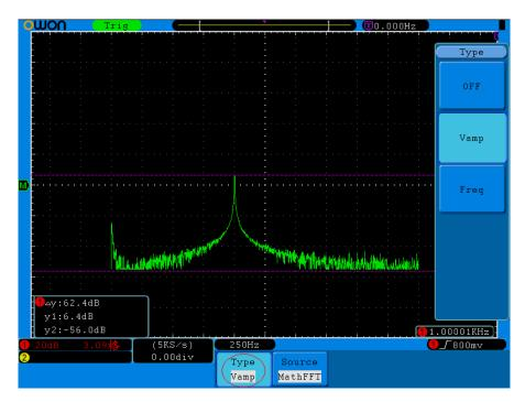
Fig.5-61 wave of Vamp cursor measurement
