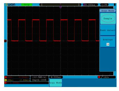
Fig.5-27 Normal ACQU Mode display, in which no burr can be detected.
