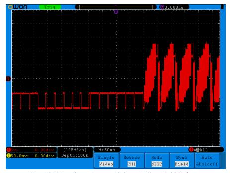
Fig.6-7 Waveform Captured from Video Field Trigger
