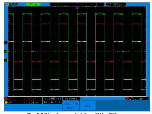
Fig. 5-7 Waveform resulted from CH1 +CH2
