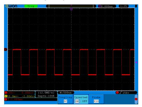
Fig. 5-5 Inverted Waveform
