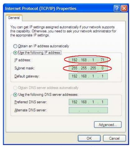
Fig.5-47 Set the network parameters of the computer
