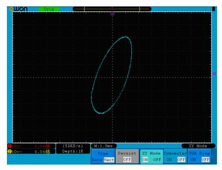
Fig.5-33 XY Display Mode
