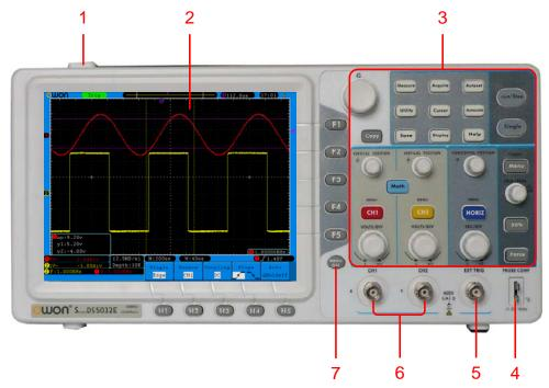
Fig. 4-1 Front panel
