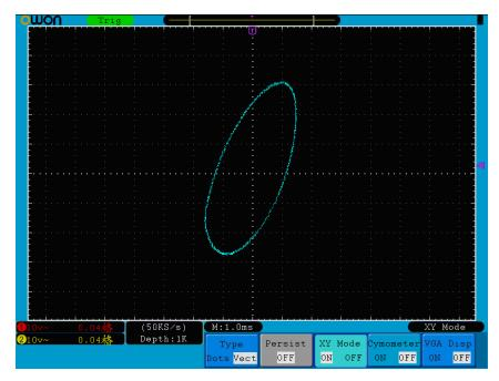
Fig.5-33 XY Display Mode
