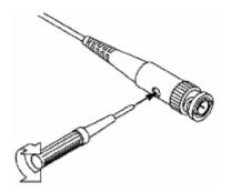
Fig. 4-9 Adjust Probe
