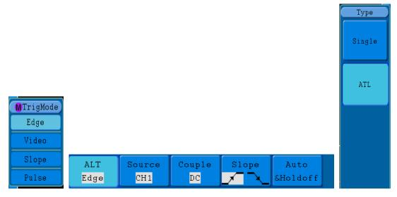
Fig.5-21 Alternate trigger (Trigger Type: Edge) Menu
