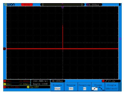
Fig.6-3 Capturing a Single Signal
