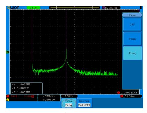
Fig.5-62 wave of Freq cursor measurement
