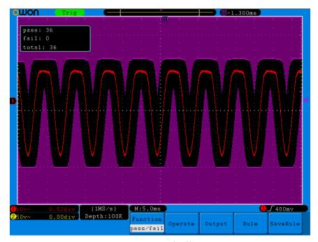
Fig.5-44 Pass/Fail test
