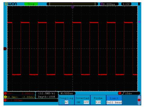
Fig. 5-2 AC Coupling Oscillogram
