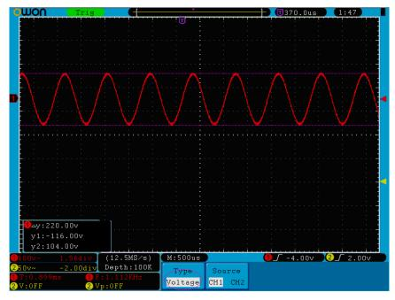
Fig.5-58 Waveform of Voltage Cursor Measurement
