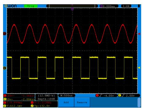
Fig.5-54 automatic measurement
