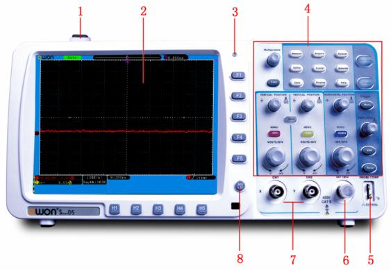
Fig. 4-1 Front panel
