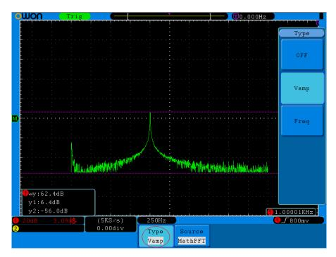
Fig.5-61 wave of Vamp cursor measurement
