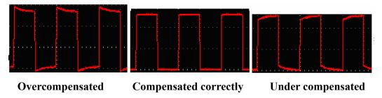
Fig. 4-8 Displayed Waveforms of the Probe Compensation
