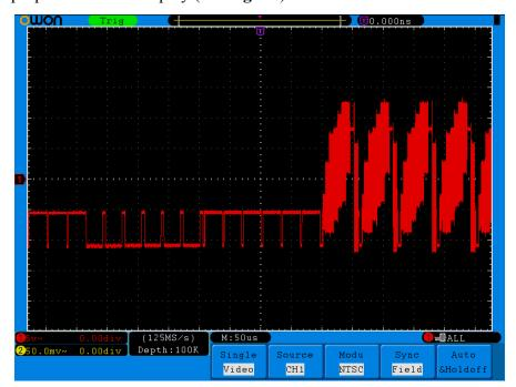
Fig.6-7 Waveform Captured from Video Field Trigger
