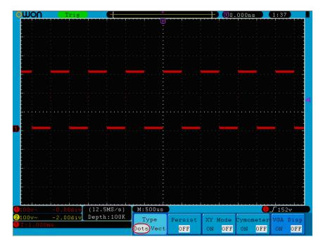
Fig.5-31 Display in Dots form
