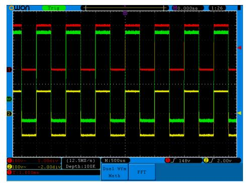
Fig. 5-7 Waveform resulted from CH1 +CH2
