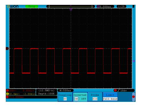
Fig. 5-5 Inverted Waveform
