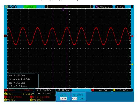
Fig.5-59 Waveform of Cursor Measurement
