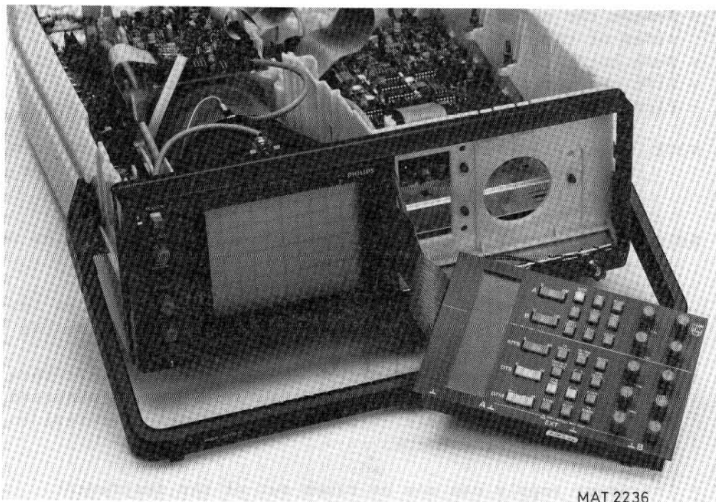
Figure 14.3 Measuring the front unit working condition
