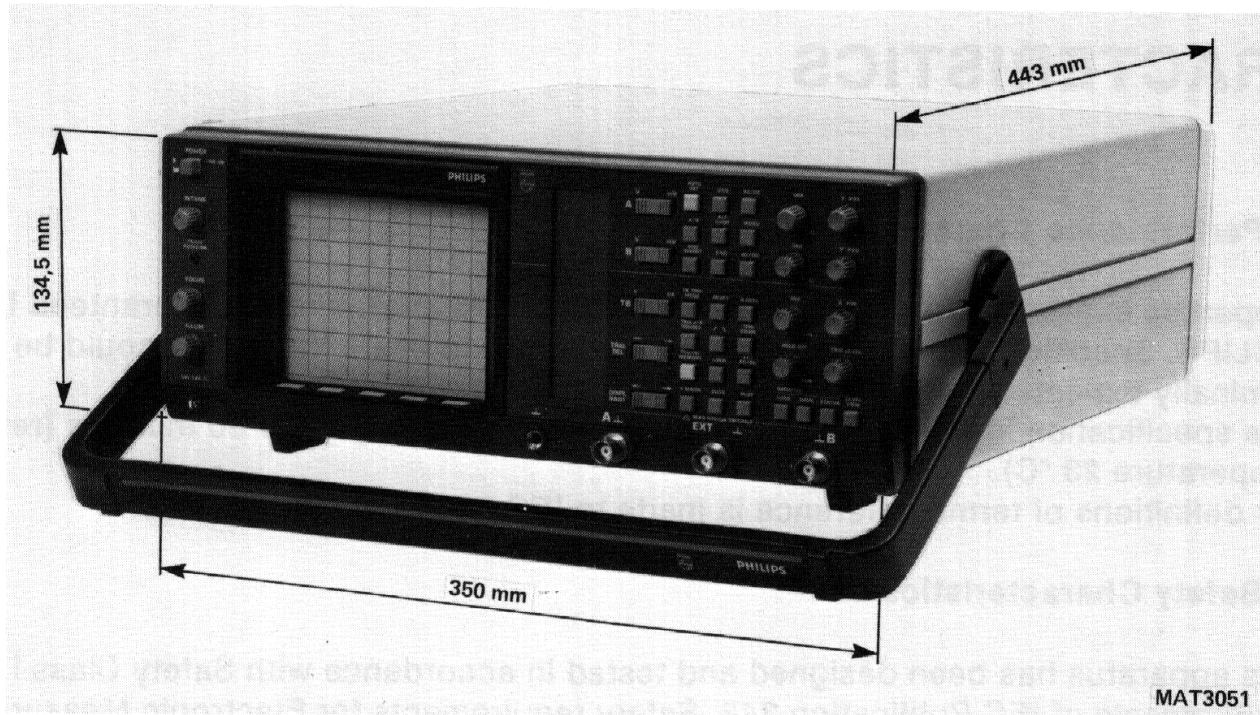
Figure 2.1 Dimensions of oscilloscope .
