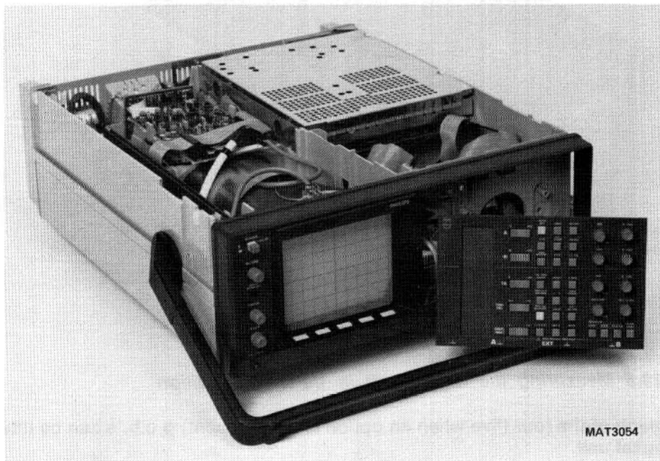
Figure 23.4 Measuring the front unit working condition
