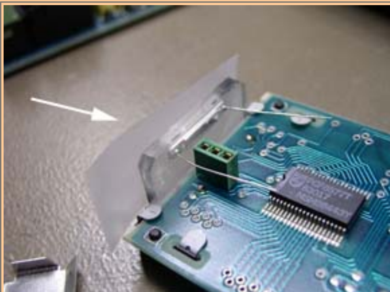
A bit of tape holds it flush for soldering, cut the
