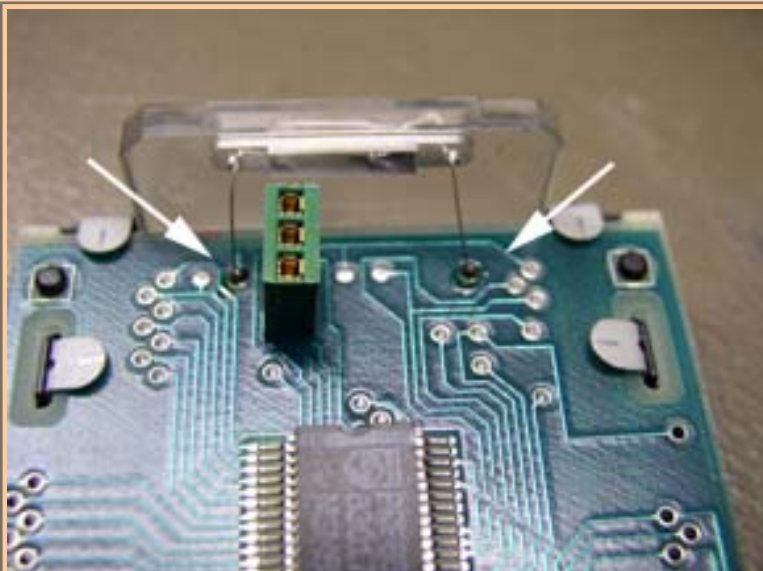
Now you need to unsolder the 2 lamp wires
