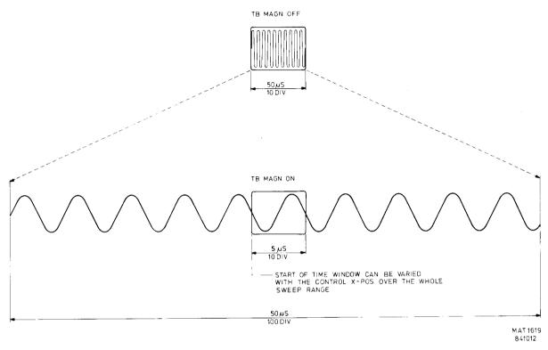
**TB MAGN**: Fixed expansion of the TIME/DIV setting by a factor of 10. Now the portion of the signal formerly displayed over a width of one division occupies the full width of the screen (10 DIV.).
