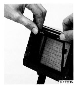
Figure 4.1 Removing the bezel and the contrast filter.
