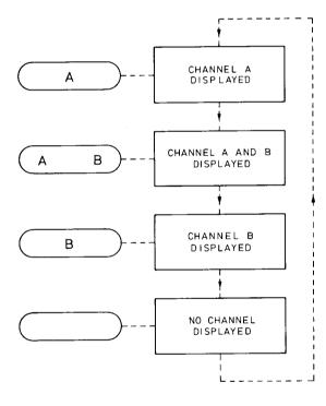
Figure 3.3 Sequence of the A/B softkey.
