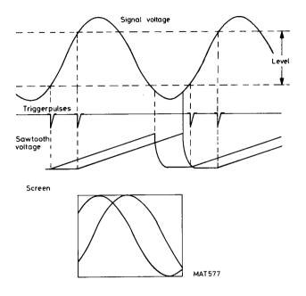
**LEVEL:** Determination of the starting point of the time-base can be varied by the LEVEL control. The time-base starts when the trigger signal reaches the voltage level of the LEVEL control.
