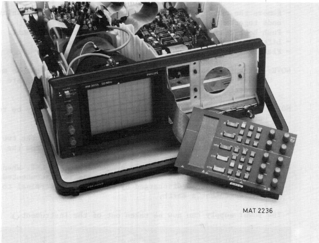
Figure 14.3 Measuring the front unit working condition
