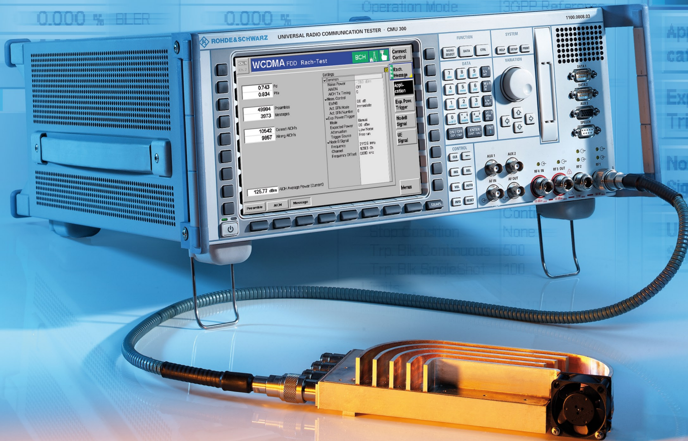
FIG 1 The R&S®CMU 300 now allows RF parameter tests to be combined with layer 1 signaling processes.
