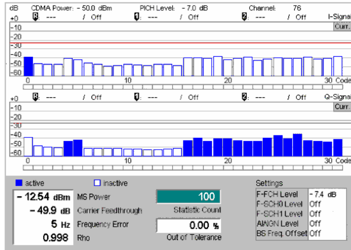
Figure 4-54 Display of measurement results (Code Domain Error Power screen)
