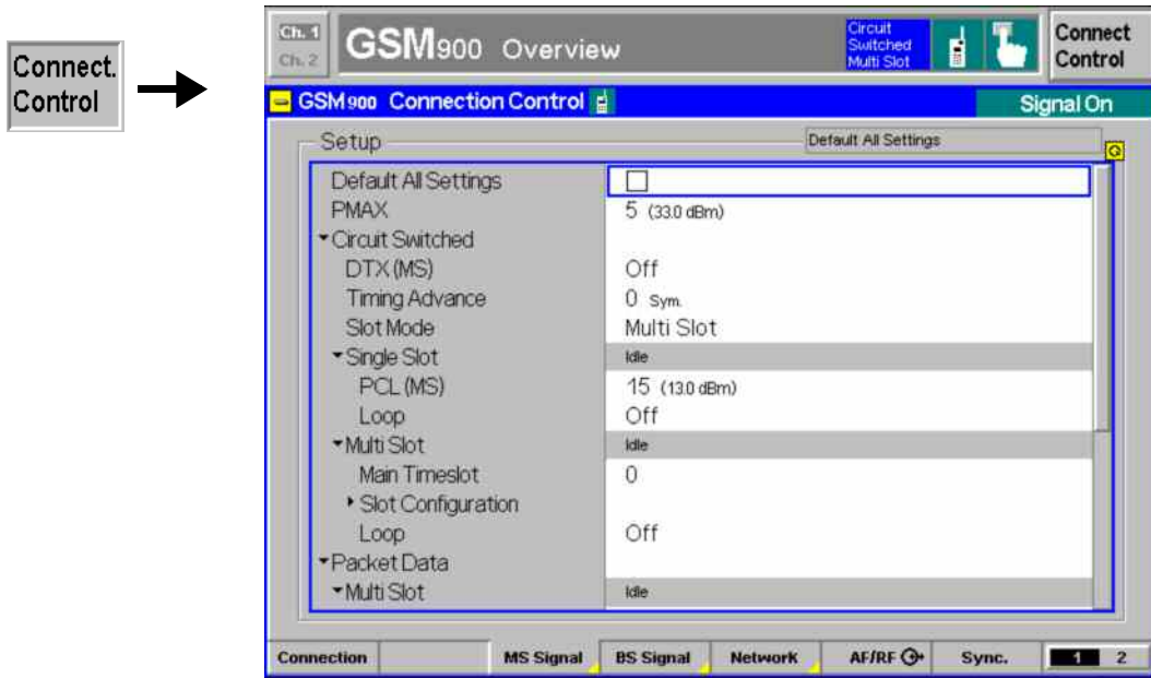
Fig. 4-105 Connection Control – MS Signal (table)
