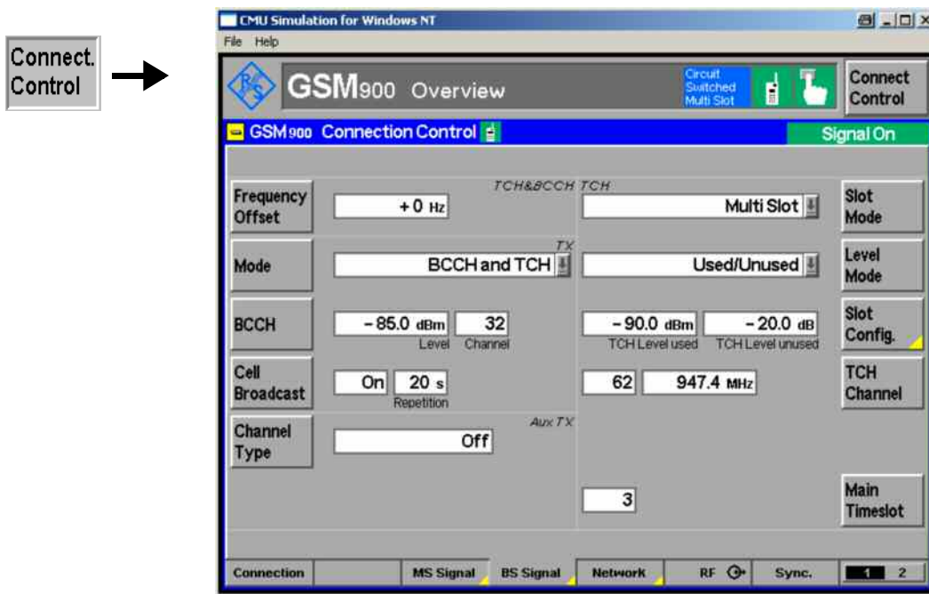
Fig. 4-107 Connection Control – BS Signal (panel, multislot)
