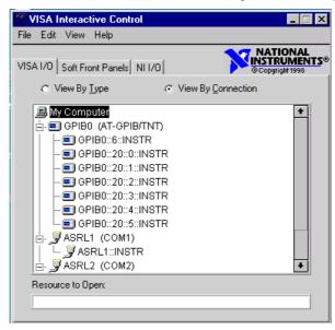
If not all devices are displayed correctly, either VISA has been installed incorrectly or there are connection problems.
