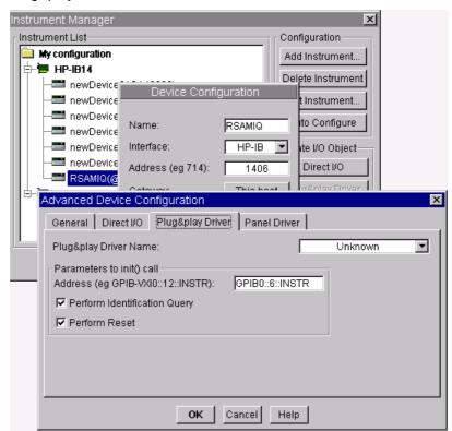
3. Click on the *Advanced I/O Config* button to open the other settings in the *Plug&play Driver* window.
