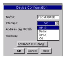
HP-IB: The measuring instrument is controlled via a GPIB card.
