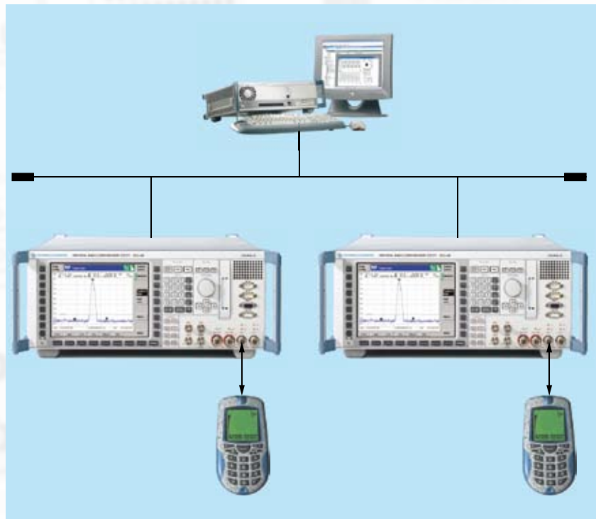
A test setup for an end-to-end test between two mobile phones for testing for problem-free MMS exchange between mobile phones from different manufacturers, for example.
