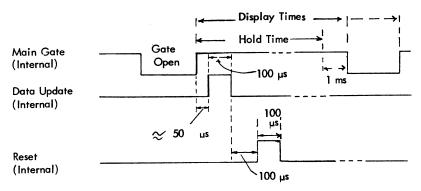
Fig. 3 Control Sequence Diagram
