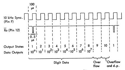
Fig. 2 Data Sequence Diagram
