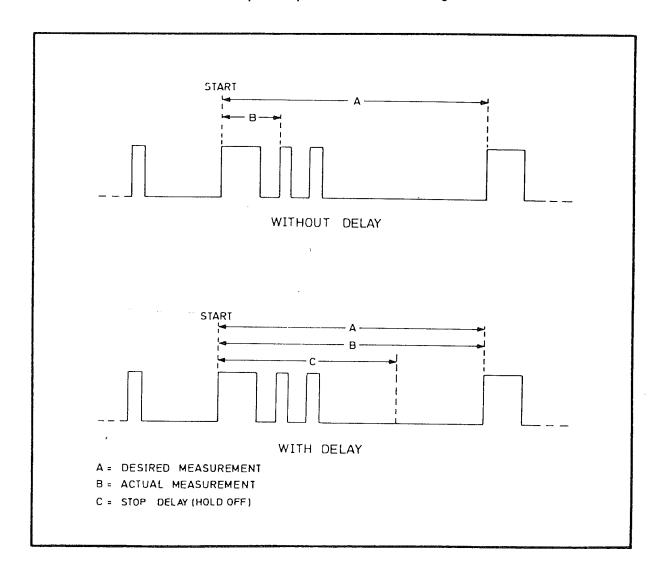
Fig 4.1 Use of Stop Circuit Delay
