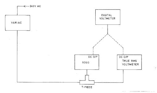
High Voltage Calibration and Input Overload Check Fig. 5.1
