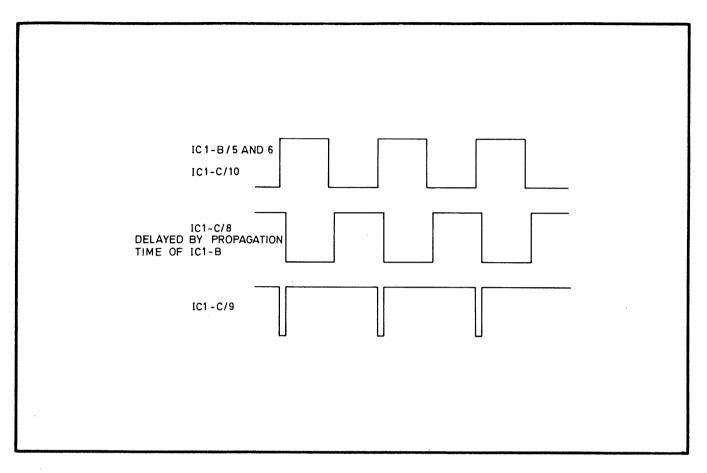
Fig. 5.2 Pulse Generator Waveforms
