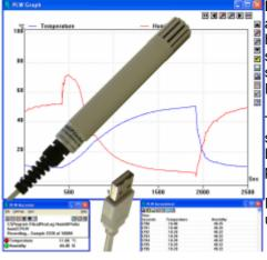
HumidiProbe is a complete, self-contained temperature and humidity measuring device. It is calibrated to give highly accurate readings, which it takes every two seconds from a dual-purpose humidity and temperature sensor. Its USB connector is compatible with standard PCs and laptops
