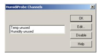
8. Double-click on **Temp unused**. The **Edit HumidiProbe Channel** dialog box appears
