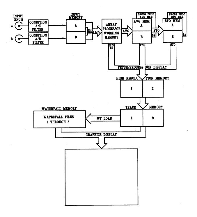
Figure A-4. SD385 Array Memory Block Diagram
