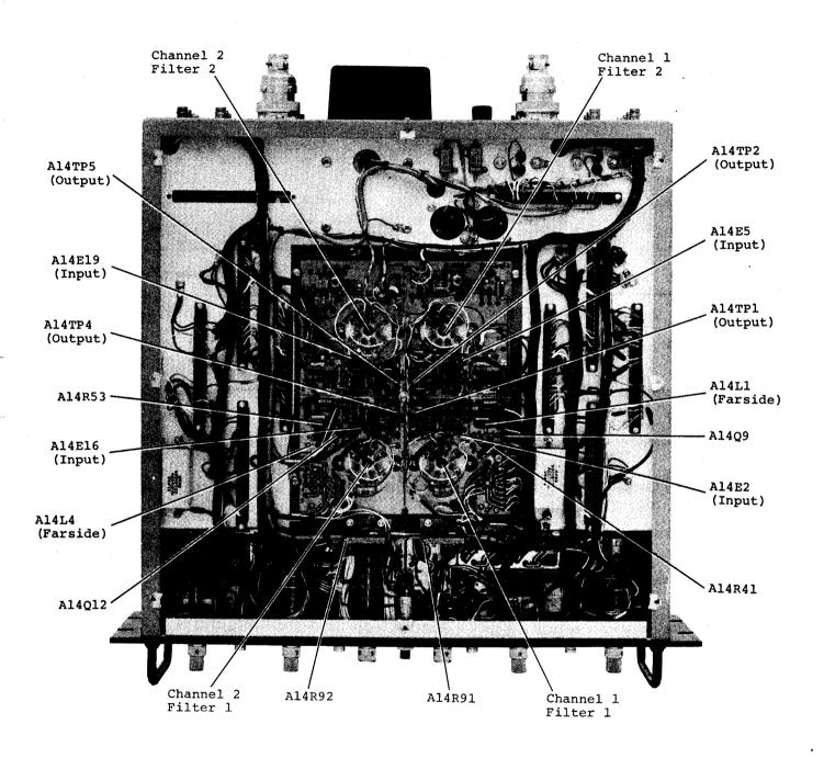
Figure 4-2. Bottom Chassis View
