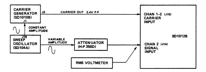
a. On the SD1010B, set the OPER/CAL switch in the OPER position and adjust the TUNING AMPL control for a centerline indication (green area) on the TUNING AMPLITUDE meter.
