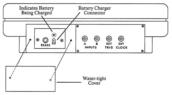
**SD222 Rear Panel Showing External Connections**
