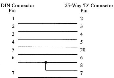
To connect to an IBM-PC computer or compatible, use a cable wired as in the following figure. This ensures correct enabling and handshaking between the devices.
