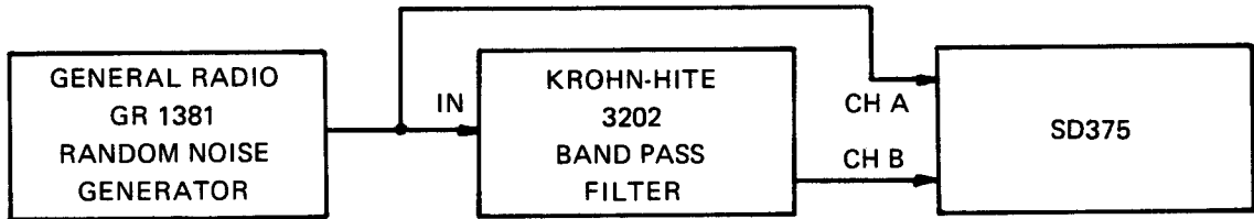
Figure 4-9. Arithmetic Function Test Equipment Interconnection
