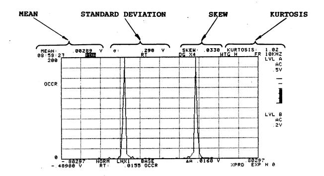
Figure 3-DSP/SEL-19. PDH Distribution of the Square Wave Shown Figure 3-DSP/SEL-18.
