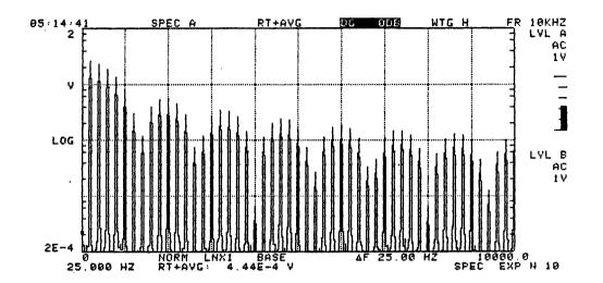
Figure 3-DSP/SEL-3. MATH FUNCTION Menu Selection 1, RT + AVG; i.e., Upper Trace, Real Time Spectrum Data Added to the Lower Trace, Average Spectrum Data
