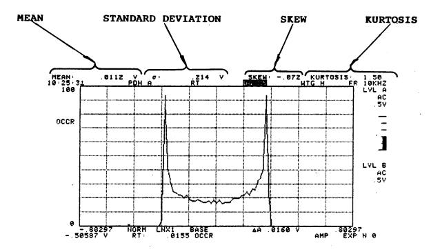
Figure 3-DSP/SEL-22. PDH Distribution of the Sine Wave Shown in Figure 3-DSP/SEL-21.
