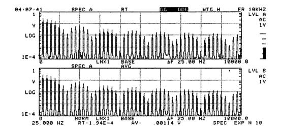
Figure 3-DSP/SEL-2. Dual-Trace, Single-Channel Display of Real Time (RT) and Averaged (AVG) Data used for the Math Operations.
