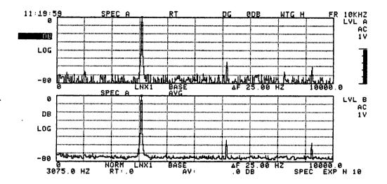
Figure 3-DSP/SEL-10. SPECTRUM FUNCTION Menu Selection 1, SPECTRUM. This is how the Lower Trace Appears after an Average is Performed.
