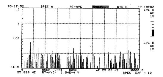
Figure 3-DSP/SEL-4. MATH FUNCTION Menu Selection 2, RT - AVG; Upper Trace, Real Time Spectrum Data i.e., Minus the Lower Trace Averaged Spectrum Data
