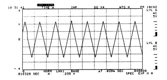
Figure 3-DSP/SEL-24. Triangle Wave Example
