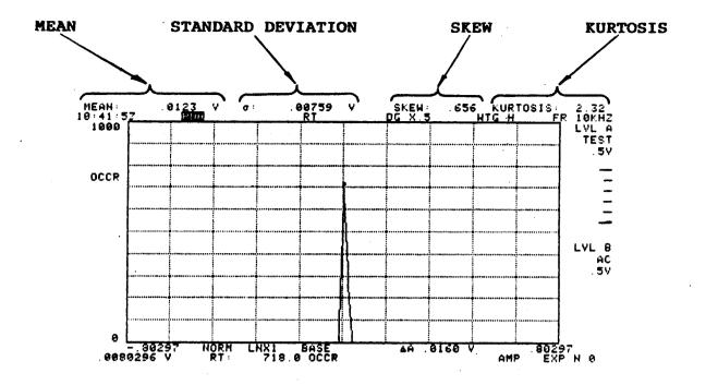
Figure 3-DSP/SEL-28. PDH Distribution of Random Noise Shown in Figure 3-DSP/SEL-27.
