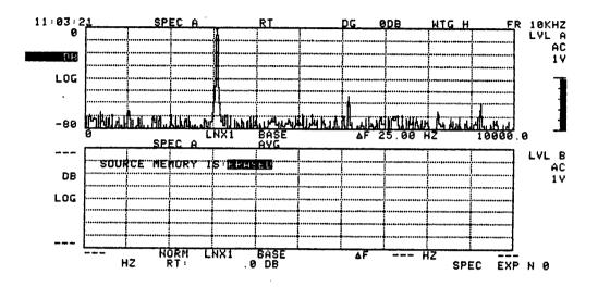
Figure 3-DSP/SEL-9. SPECTRUM FUNCTION Menu selection 1, SPECTRUM This is how the Lower Trace Appears before an Average is Performed.
