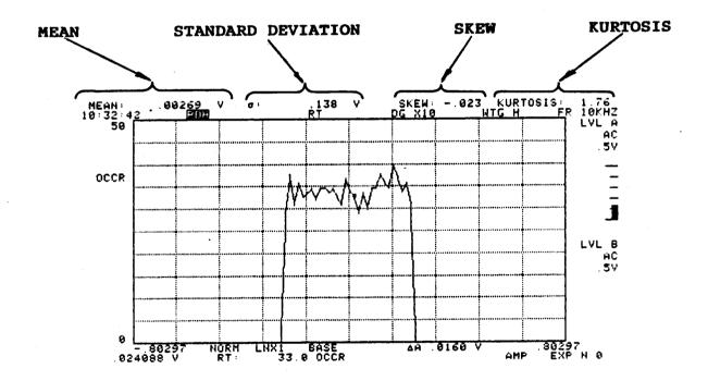
Figure 3-DSP/SEL-25. PDH Distribution of Triangle Wave Shown in Figure 3-DSP/SEL-24.
