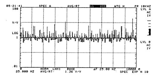
Figure 3-DSP/SEL-8. MATH FUNCTION Menu Selection 6, AVG/RT; i.e., Lower Trace, Averaged Spectrum Data Divided by the Upper Trace, Real Time Spectrum Data
