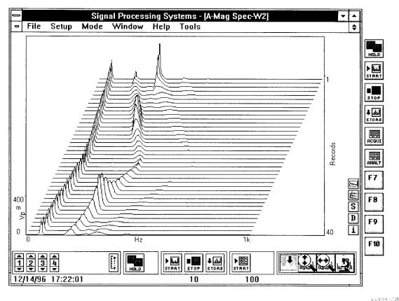
Hidden line removal is always enabled for cascade displays. Selectable amplitude of a single trace, the number of traces to display, skew, and baseline suppression can enhance the viewing of cascaded data.
