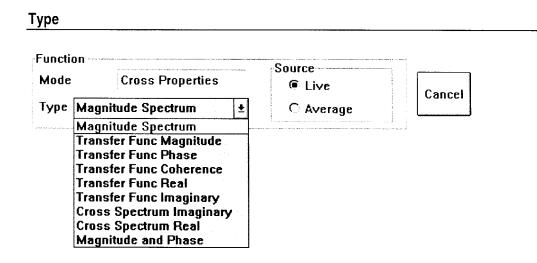
This is a pull-down combo box displaying the types of functions that can be loaded into waterfall memory for the selected mode. Only one function can be selected. The selected function applies to all active channels selected in the **Setup Waterfall Input** group. If a **Magnitude Spectrum** waterfall is selected for **Channel 1**, then other active channels for which a waterfall display is selected must also display a magnitude spectrum waterfall.
