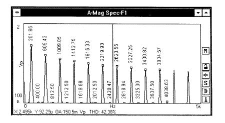
If frequency interpolation is activated before selecting **Harmonic** Markers, the marker "dots" will often line up exactly on the harmonic peaks and no further "fine tuning" is necessary. If fine tuning is necessary, note that alignment of the markers is done with sub-bin resolution.
