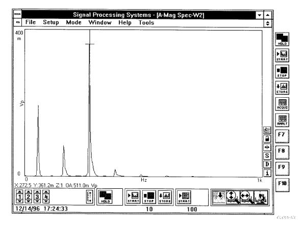
This display type will display a single trace from waterfall memory. It is an accurate representation of the most recent data being loaded into waterfall memory during **Live** load. During waterfall data recall, any individual record can be displayed from waterfall memory by prompting the waterfall icon, located in the display control totem pole to the right of the trace border, and making a record selection.
