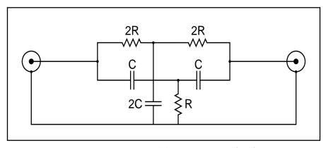
Figure 6-1 Twin-Tee Notch Filter
