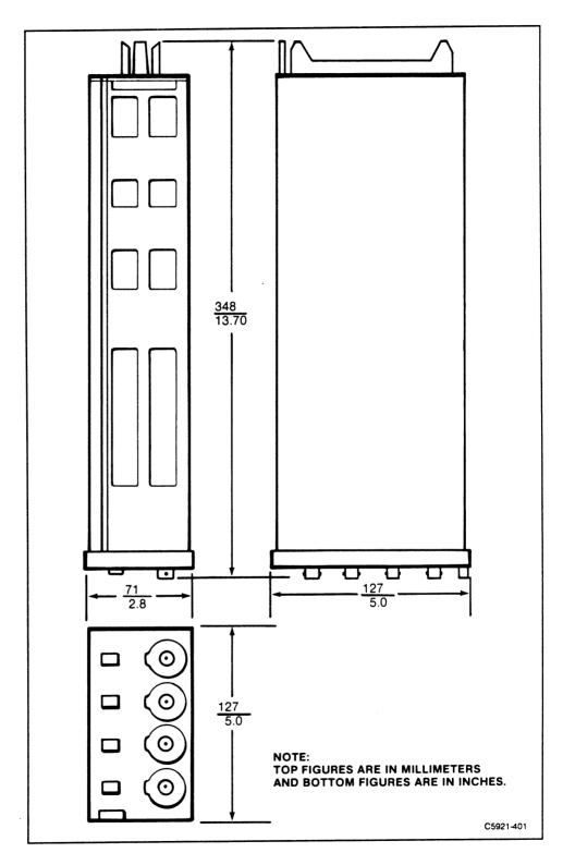
Figure 4-1. Dimensions of 11A34.
