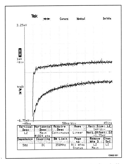
Figure 3-2. Overdrive recovery using short (top) and long (bottom) cables terminated in  $50\,\Omega$ . Traces are offset two divisions and the illustration is a composite of two waveforms.
