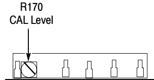
Figure 5-7: CAL Level Adjustment on Reference Oscillator Board
