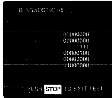
TYPICAL FAILURE DISPLAY FOR TEST 5. REFER TO FIGURE 21.
