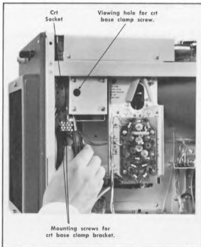
Fig. 4-3. Loosening the crt base clamp.
