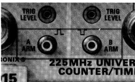
Fig. 1 Measuring the time interval between two non-adjacent pulses using trigger arming.
