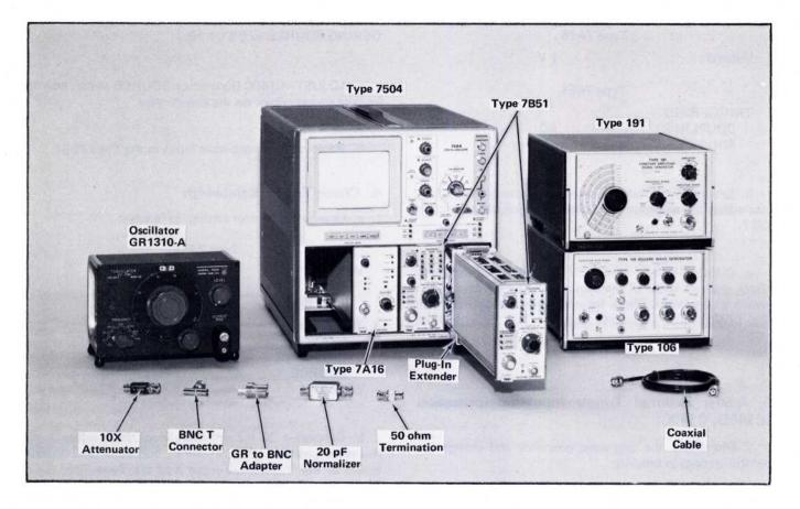
Fig. 5-1. Test equipment required for steps 1 through 8.
