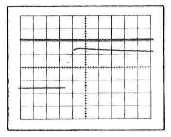
Fig. 5-11. Typical CRT display showing delay time jitter.
