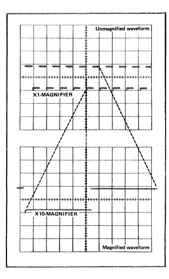
Fig. 2-9. Operation of sweep magnifier,
