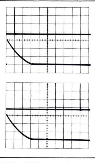
Fig. 5-10. Typical CRT display showing delay adjustments correctly set.
