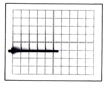
Fig. 5-4. Typical CRT display when checking sweep length.
