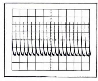
Fig. 5-7. CRT display showing correct .2 µs timing.
