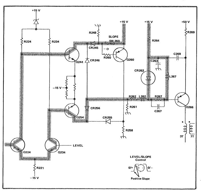
Fig. 3-4. Trigger Path for Positive Slope Triggering (simplified).
