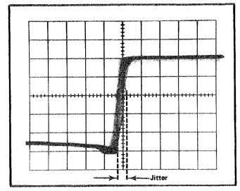
Fig. 2-15. Measuring pulse jitter.
