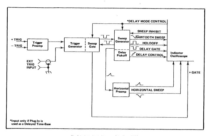
Fig. 3-1. Basic Block Diagram of the Type 7B51.
