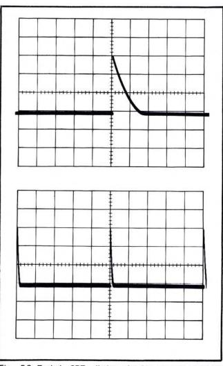
Fig. 5-3. Typical CRT display showing correct magnifier registration. (A) MAGNIFIER set to X10, (B) MAGNIFIER set to X1.
