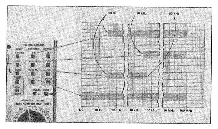
Fig. 2-6. Frequency range of each COUPLING switch position.
