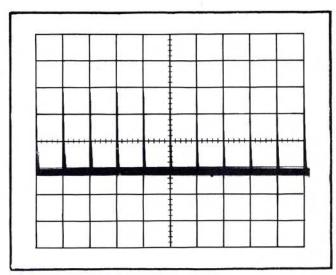
Fig. 5-2. Typical CRT display showing correct sweep calibration.
