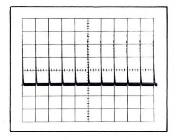
Fig. 5-6. CRT display showing correct 5 µs timing.
