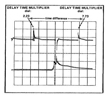
Fig. 2-12. Measuring time difference using delayed sweep.
