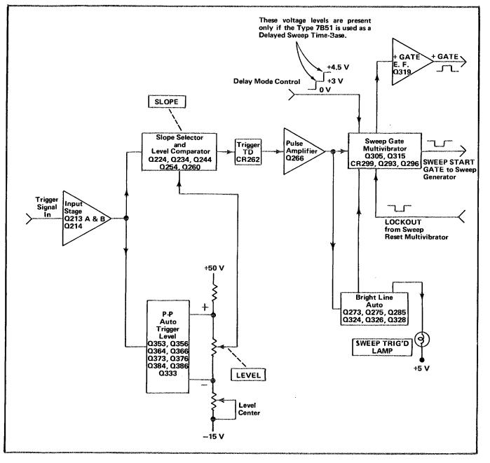
Fig. 3-3. Trigger Generator Block Diagram.
