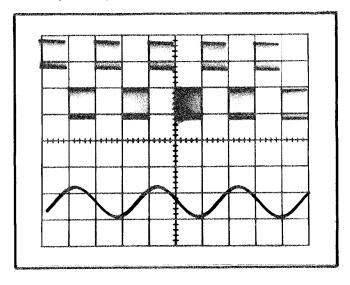
Fig. 2-14. Displaying a complex signal using delayed sweep.
