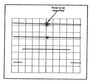
Fig. 2-13. Using delayed sweep for sweep magnification.
