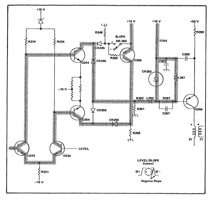
Fig. 3-5. Trigger Path for Negative Slope Triggering (simplified).
