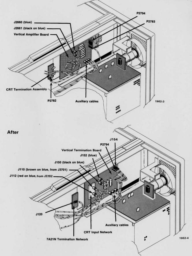
Fig. 6. Shows board positions and cable connections before and after installation of 7A21N in the 7844; right side, Beam 2. @
