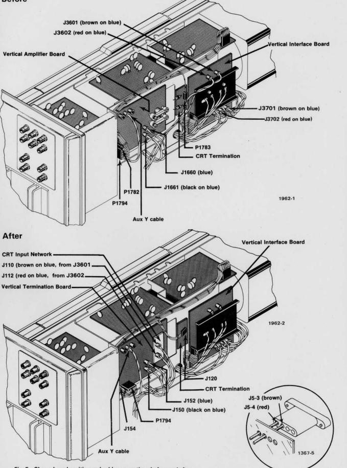
Fig. 5. Shows board position and cable connections before and after installation of 7A21N in the 7844; left side, Beam 1.
