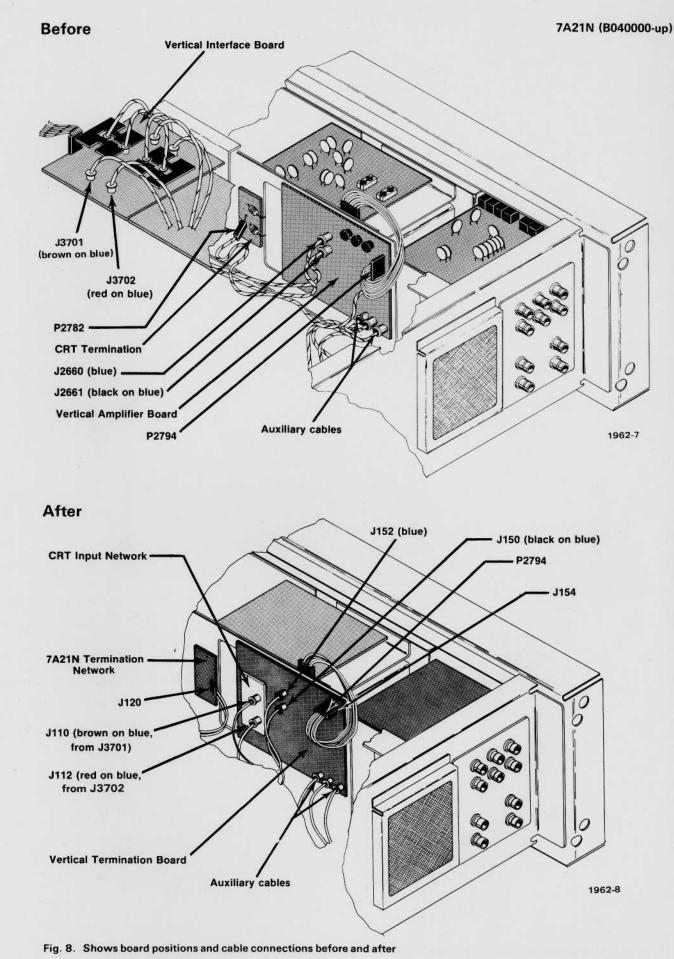
installation of 7A21N in the R7844; right side, Beam 2.
