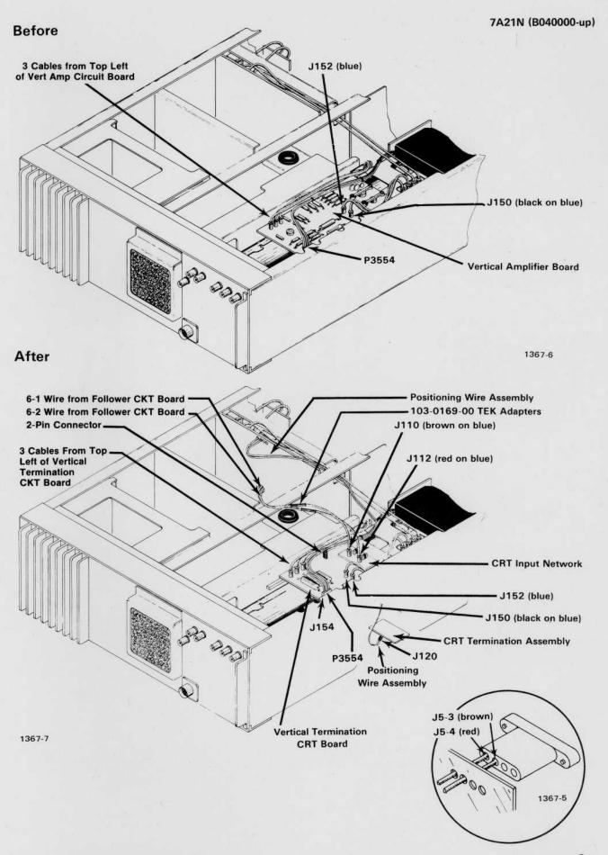
Fig. 11. Shows board positions and cable connections before and after installation in the R-7912.
