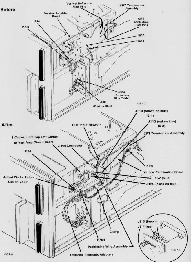
Fig. 10. Shows board positions and cable connections
