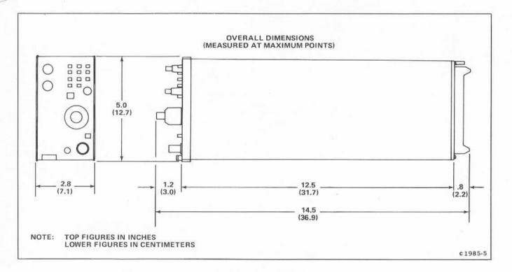
Figue 1-2. 7B15 dimensional drawing.
