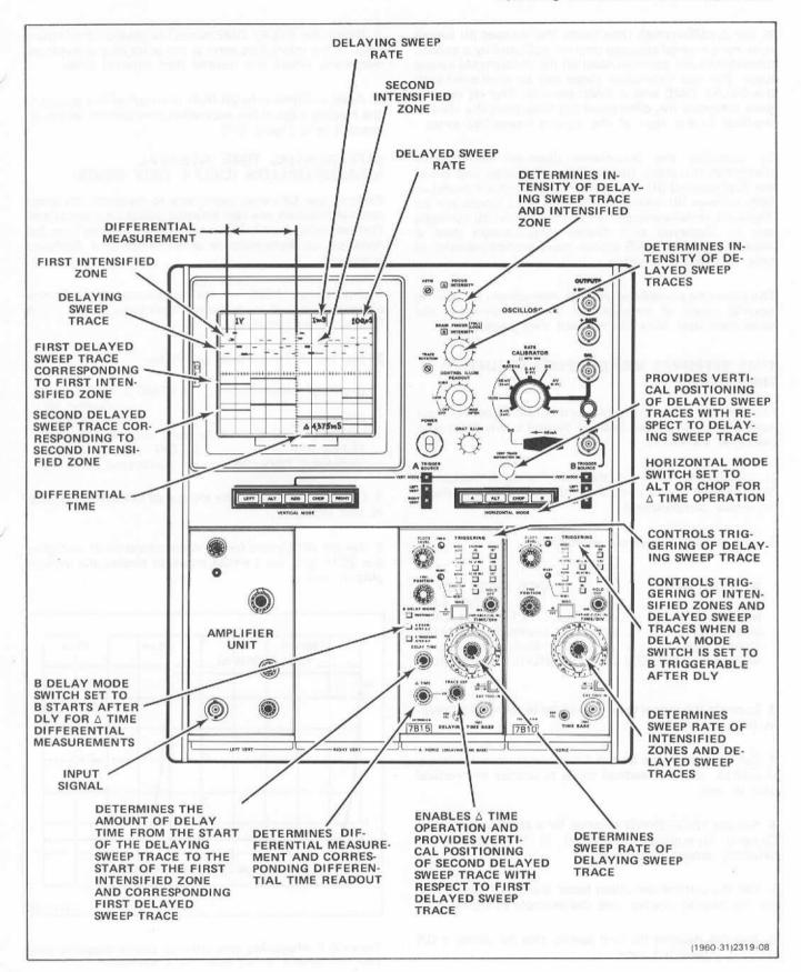
Figure 2-6. Typical  $\triangle$  (Differential) Time Operation.
