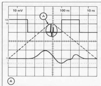
THIS PORTION OF THE DISPLAY CANNOT NORMALLY BE EXAMINED IN DETAIL BECAUSE THE DELAYING (A) SWEEP IS TRIGGERED ON THE LARGER AMPLITUDE SIGNALS AT THE START OF THE DISPLAY.
