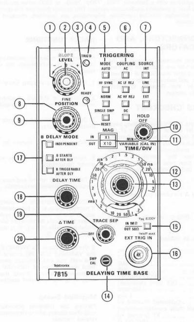
Figure 2-1. Front-panel controls, connectors and indicators.
