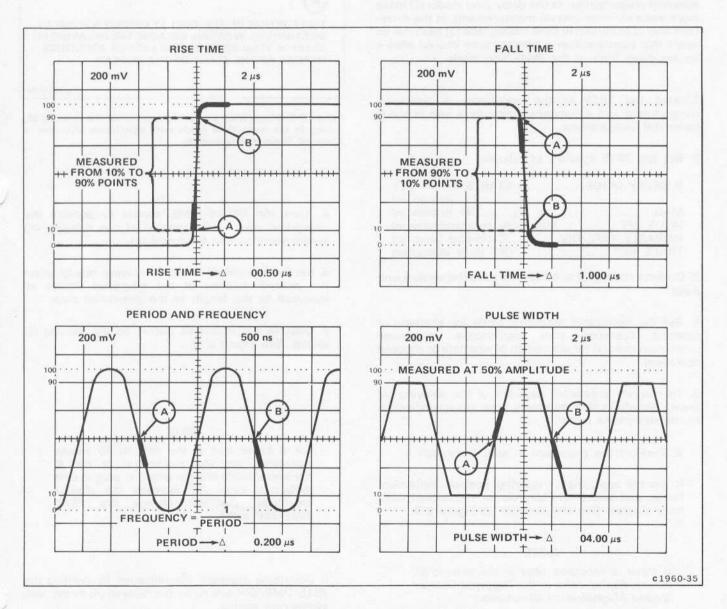
Figure 2-8. Measuring risetime, fall time, period, frequency, or pulse width in the \( \triangle \) (differential) time mode.
