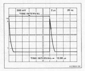
Figure 2-7. Measuring time intervals from a triggering event (start of sweep) to any point on a waveform.
