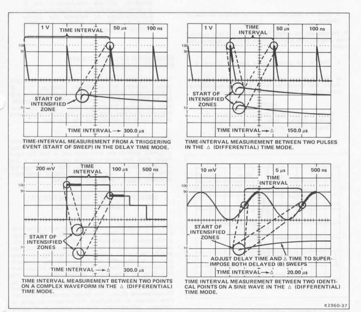
Figure 2-10. Time-interval measurements in the delay-time and  $\triangle$  (differential) time mode with mainframe alternate or chopped operation.
