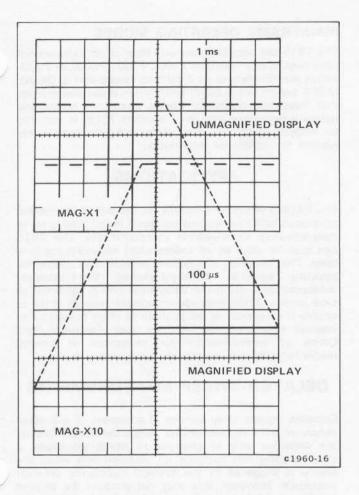
Figure 2-4. Effect of sweep magnifier on crt display.
