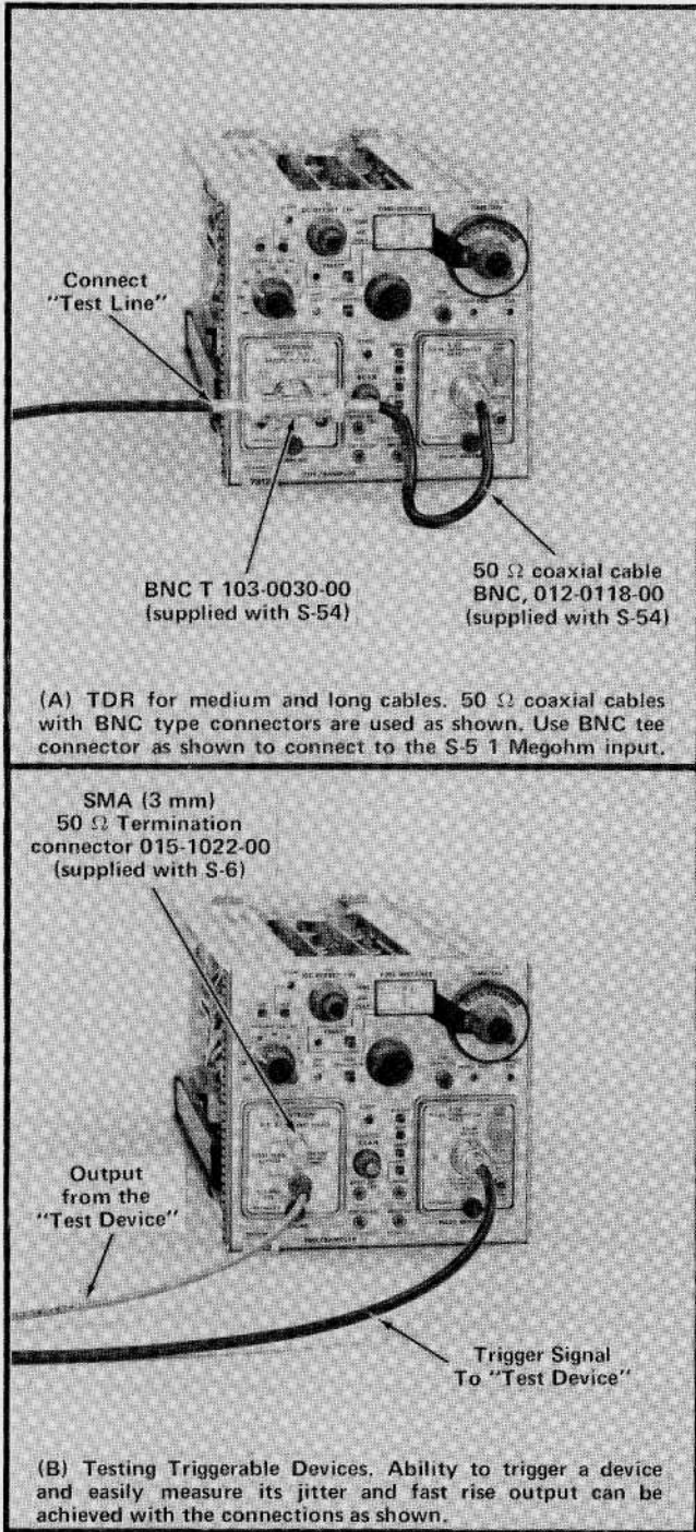
Fig. 2-11. Application connections (A) for TDR of medium and long cables and (B) for testing triggerable devices.
