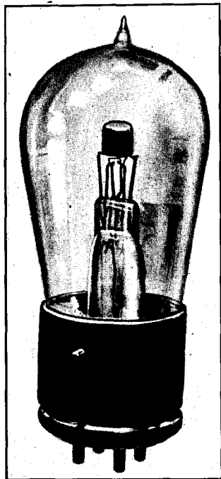
FIG. 130.—General Electric type Receiving Tube. Length: 10 cms.
