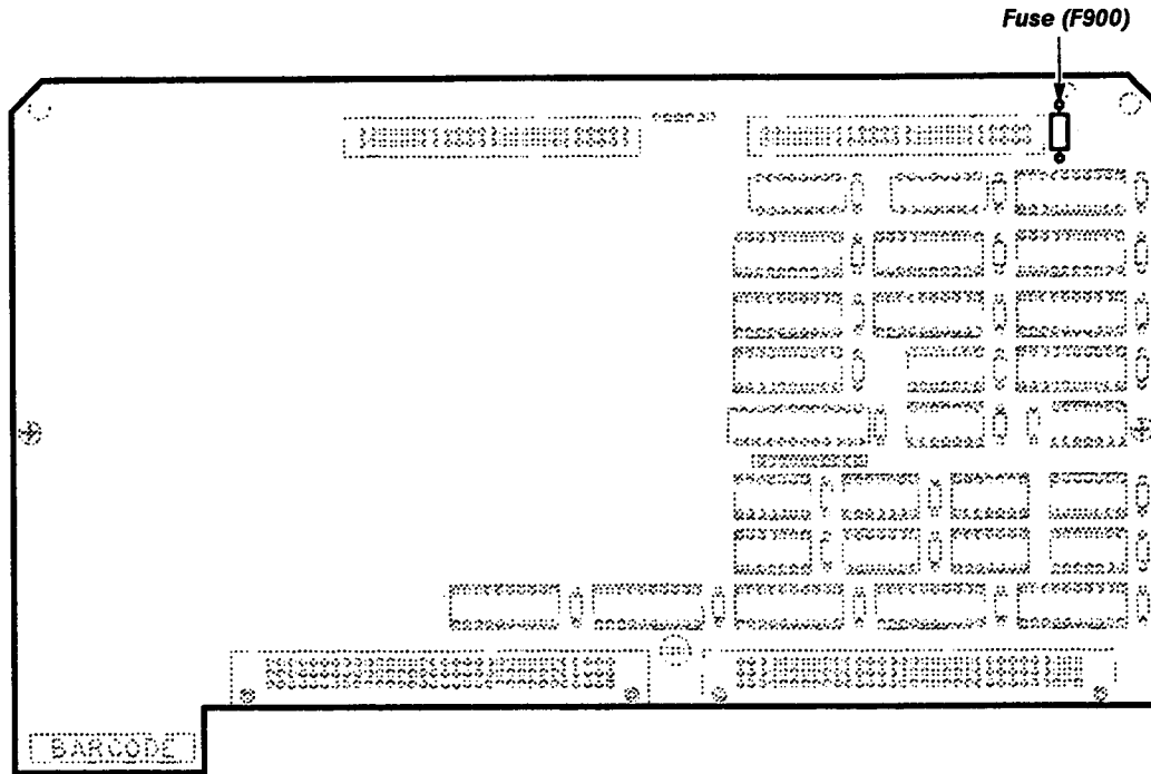
Figure 3-8 — A20 Digitizer I/O Board Fuse Locator Diagram
