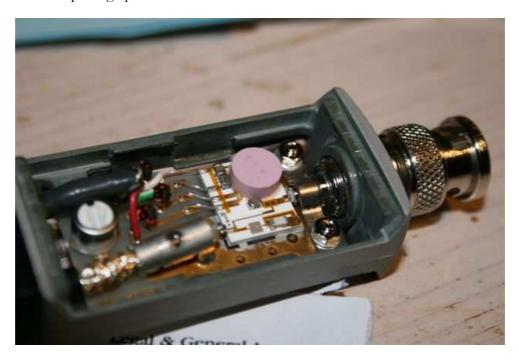
The basic design is an RF power splitter, and a voltage doubler peak detector. The diodes for the detector are under the pink isothermal cover at the top right of the hybrid, as are the reference diodes and a few other components.
