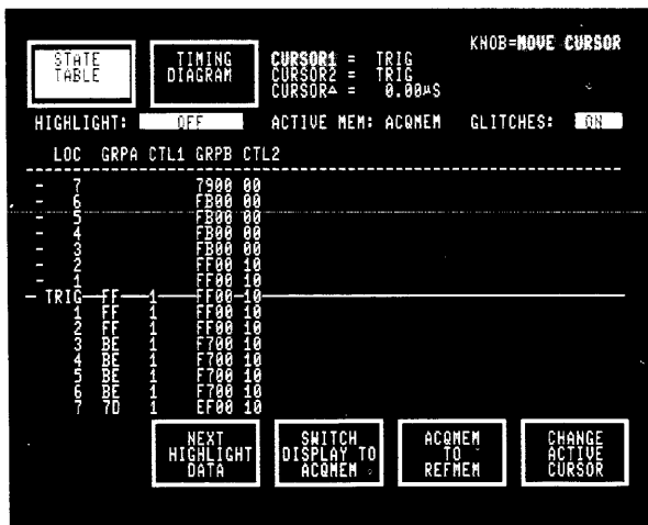
Figure 2-3. Data acquired at 20 ns ASYNC after triggering on FF in the TPG pattern.
