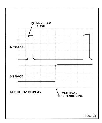
Figure 4-13. Time difference between repetitive pulses.
