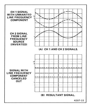
Figure 4-5. Common-mode rejection.
