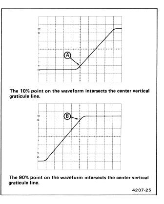
Figure 4-15. Rise time, differential time method.
