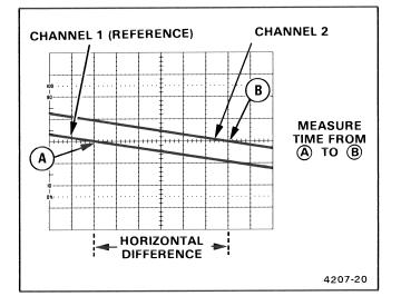
Figure 4-10. High-resolution phase difference.
