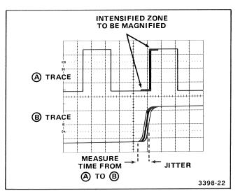
Figure 4-12. Pulse jitter.
