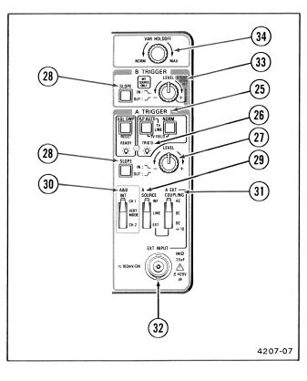
Figure 2-6. Trigger controls, connector, and indicator.
