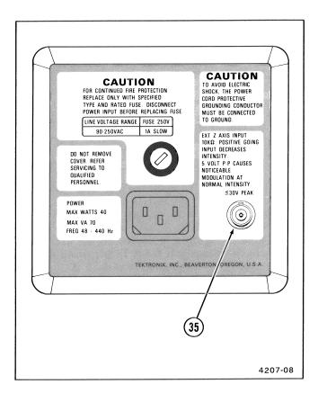
Figure 2-7. Rear-panel connector.
