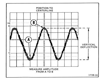
Figure 4-2. Peak-to-peak waveform voltage.
