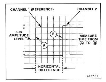
Figure 4-8. Time difference between two time-related pulses.
