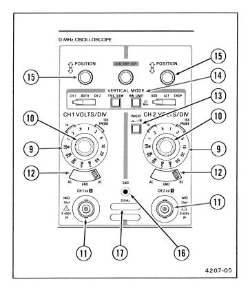
Figure 2-4. Vertical controls and connectors.
