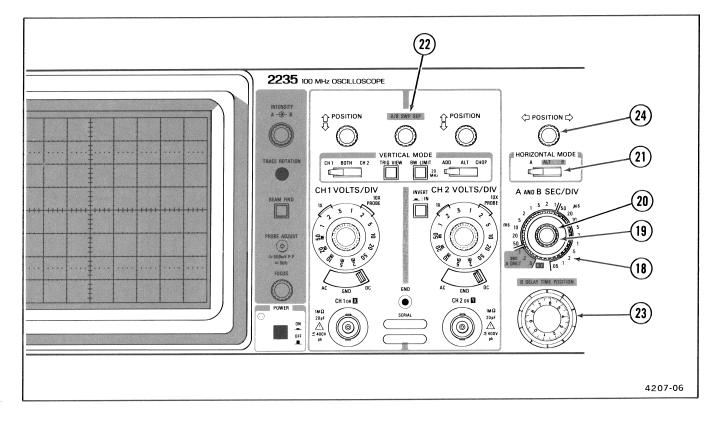
Figure 2-5. Horizontal controls.
