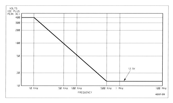
Figure 1-1. Maximum input voltage vs frequency derating curve for CH 1 OR X, CH 2 OR Y, and EXT INPUT connectors.
