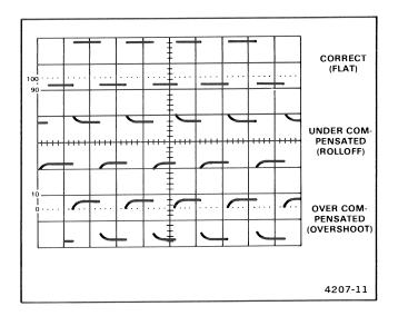
Figure 3-2. Probe compensation.
