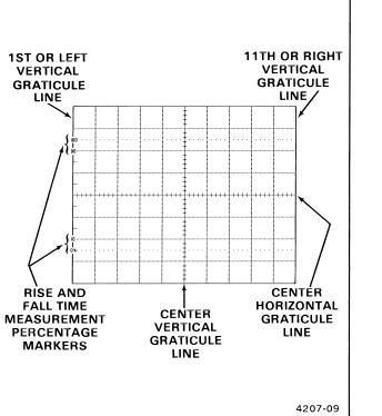
Figure 3-1. Graticule measurement markings.
