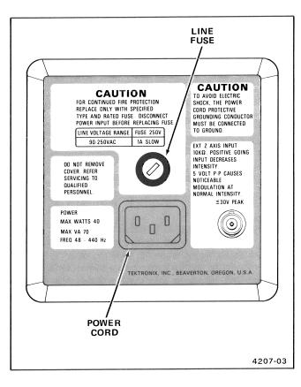
Figure 2-2. Fuse holder and power cord connector.
