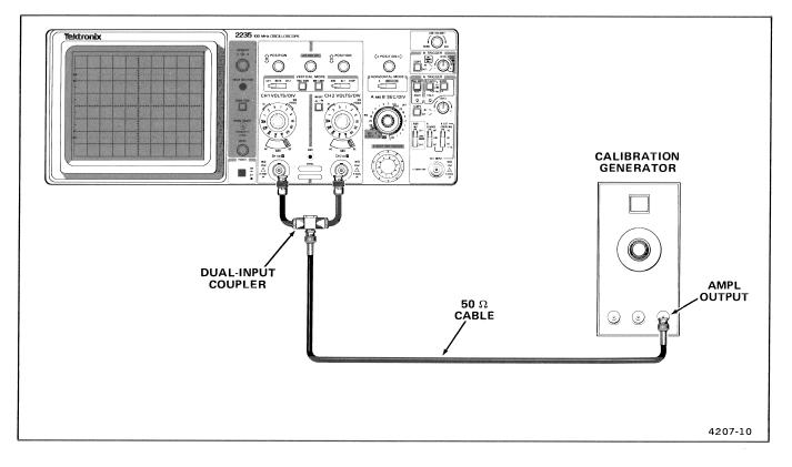
Figure 4-1. Initial setup for instrument familiarization procedure.
