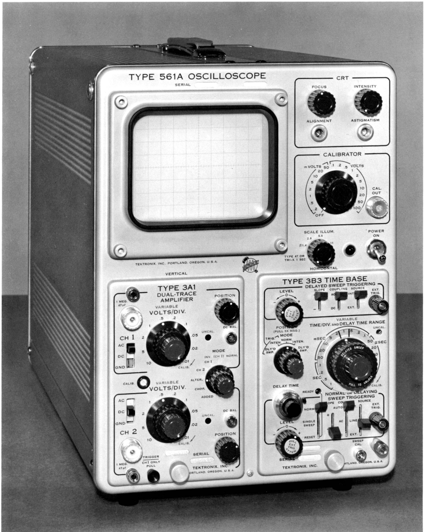
The Type 561A Oscilloscope, including the Type 3A1 Dual-Trace Amplifier and the Type 3B3 Time Base.
