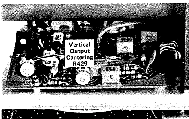
Fig. 5-9. Location of Vertical Output Centering adjustment.
