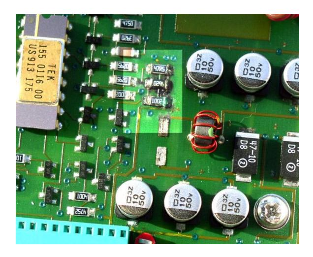
The black "crud" in the highlighted area doesn't originate from the resistors or from the soldering or assembly process. Rather, it's caused by outgassing of corrosive vapors from one or more of the 10 uF/50V electrolytics nearby. Any corroded traces should be cleaned or bridged as soon as you spot the problem, and *all* of the aluminum-can electrolytics should be replaced.
