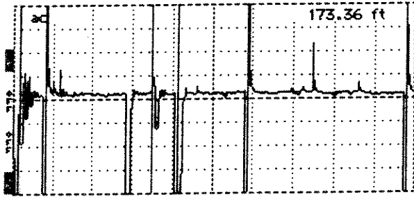
1A - Tap hidden by traffic (1 avg, 50 ft/DIV, 35.00 dB gain)
