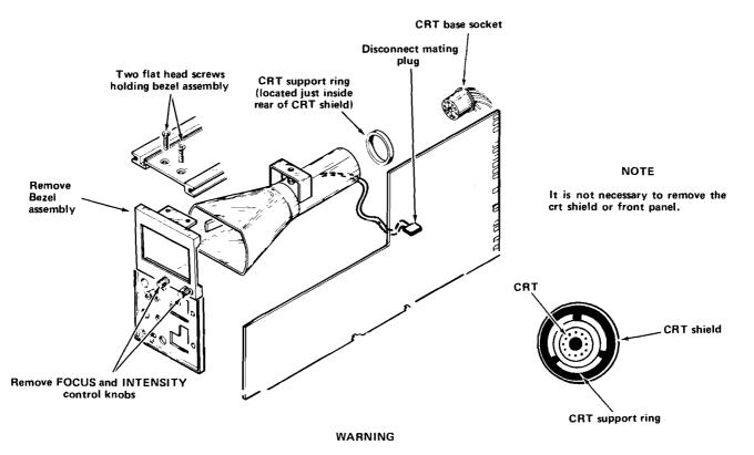
Use care when handling a crt. Protective clothing and safety glasses should be worn. Avoid striking it on any object which might cause it to crack or implode. When storing a crt, place it in a protective carton or set it face down in a protected location on a smooth surface with a soft mat under the faceplate to protect it from scratches.
