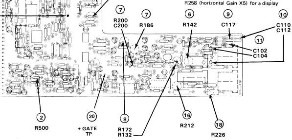
of two time marks per five major divisions. Position display horizontally from full left to full right. Signal linearity must remain within ±2 minor divisions. Return horizontal POSITION control to midrange. Push time base VARIABLE control in and set to X1 position.
