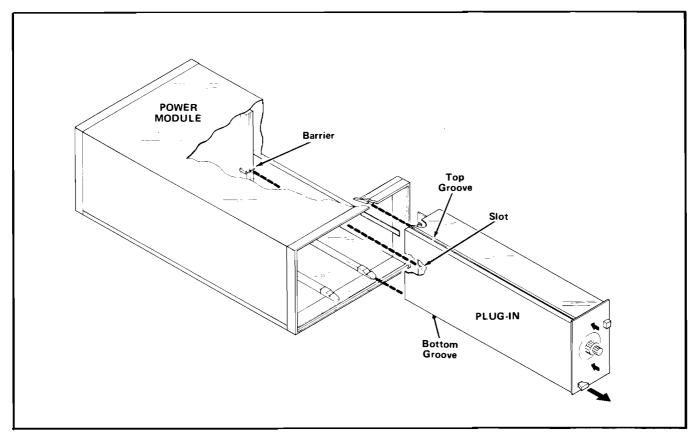
Fig. 1-1. Plug-In Installation and removal.
