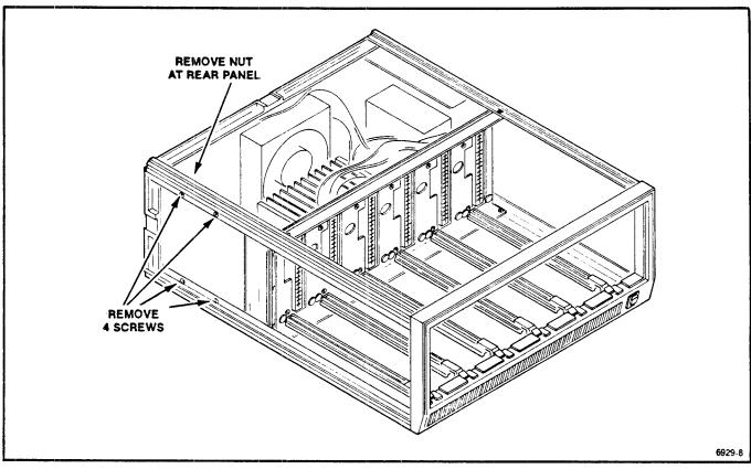
Fig. 3-6. Location of screws holding the dc power supply circuit board to the mainframe chassis.
