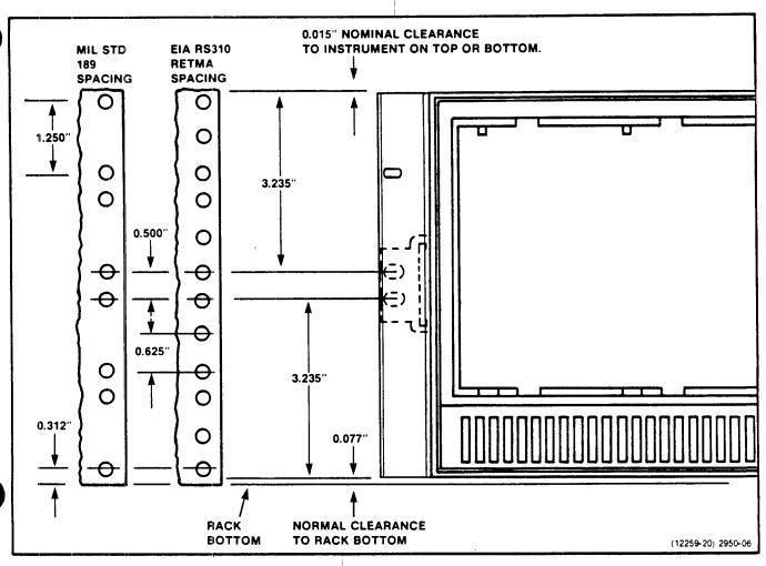
Fig. 2-6. Dimensions and positioning of TM 506A, Option 10, in standard rack.
