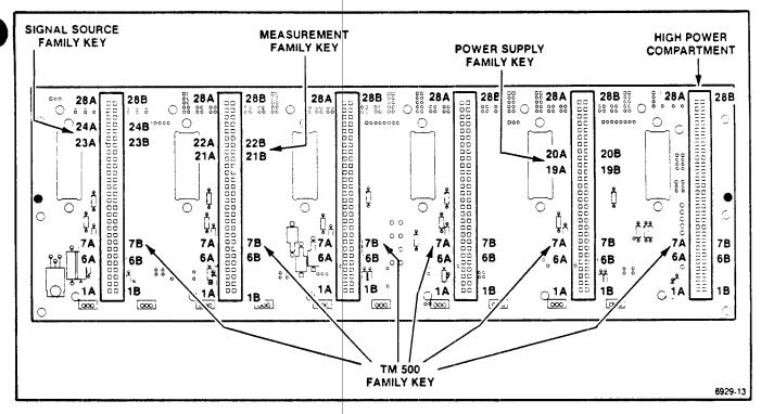
Fig. 2-11. Keying assignments for family functions. One of the many possible sequence combinations.
