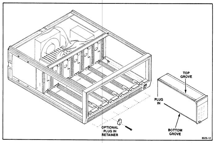
Fig. 2-10. Plug-in installation and removal.
