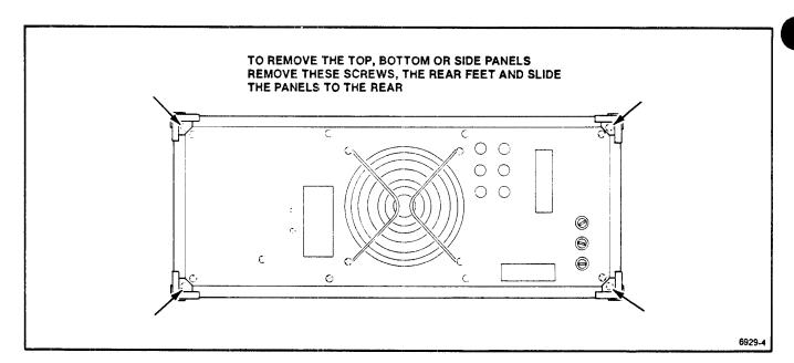
Fig. 3-2. Outer panel removal.
