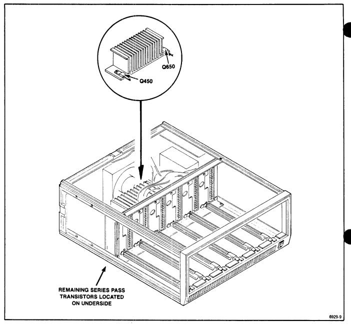
Fig. 3-7. Series pass transistor locations. The high power compartment series pass transistors Q450 and Q650 are on the right side of the heat sink. Q650 is the upper transistor.
