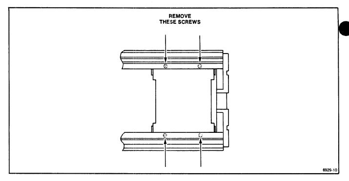
Fig. 3-9. Transformer assembly attaching screws.
