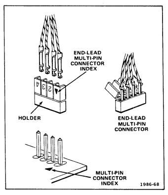
Fig. 3-1. Orientation and disassembly of multipin connectors.
