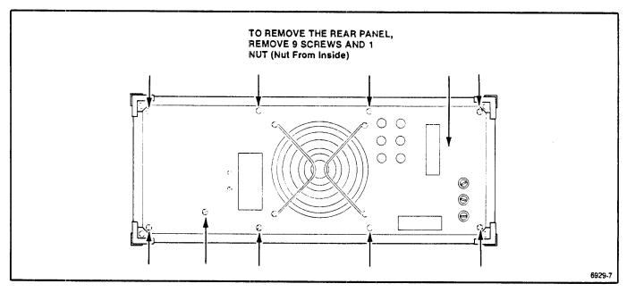
Fig. 3-5. Rear panel removal.
