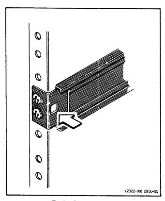
Fig. 2-5. Rack latch hole.
