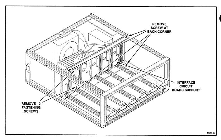
Fig. 3-4. Removal of the interface circuit board support.
