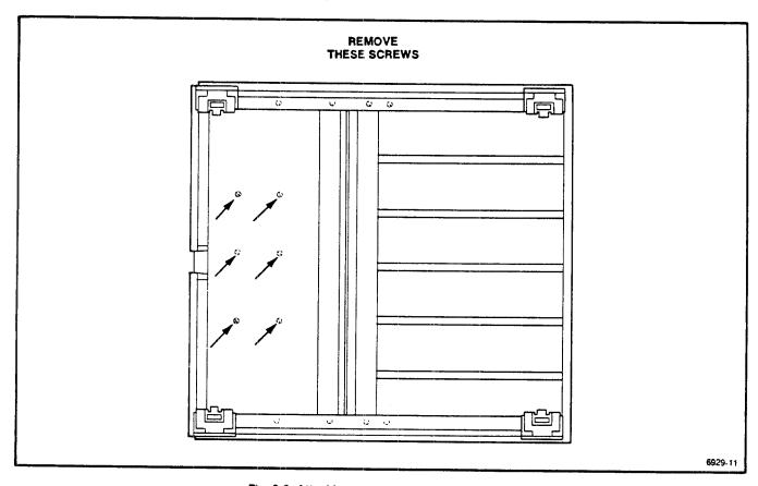
Fig. 3-8. Attaching screws on bottom of mainframe.
