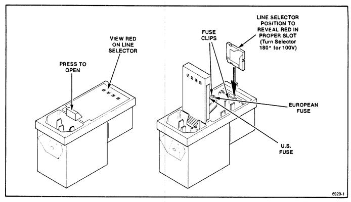
Fig. 2-1. Line Voltage Selection and Main Fuse Replacement.
