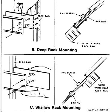
Fig. 2-8. Rackmounting slide details.
