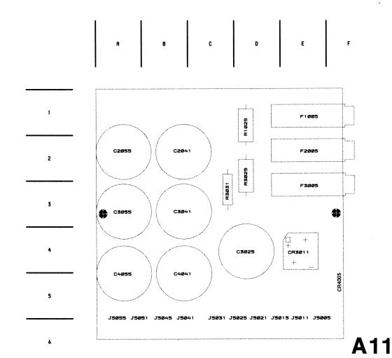
Fig. 6-2. A11—Power Supply circuit board assembly.
