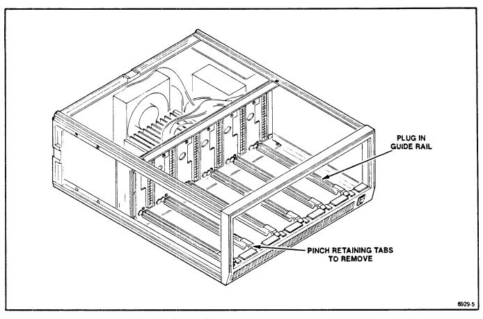
Fig. 3-3. Guide rail and air baffle removal.
