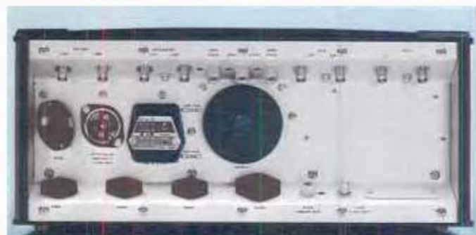
Fig 8—Rear view of 520 Vectorscope. The mounting angle of the coax connectors permit connecting cables to leave the instrument without protruding excessively and with a minimum of clearance space required.
