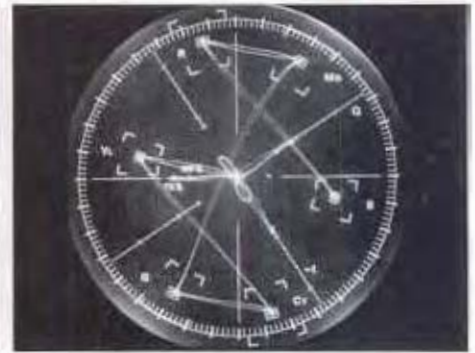
Fig 15: Vector display. Split field color bars, 75% amplitude, 100% white reference, 10% setup. Conforms to EIA specification RS 189.
