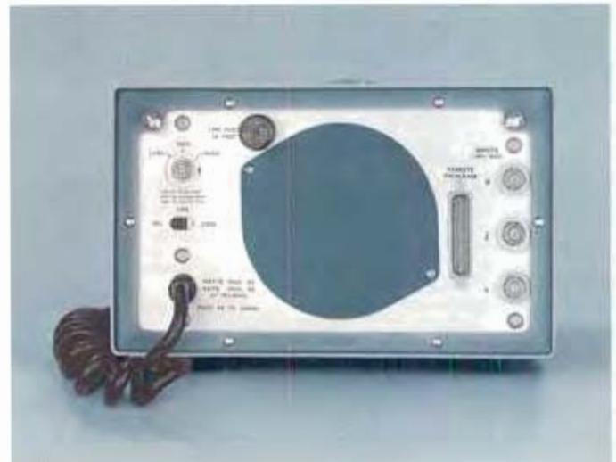
Rear panel of Type 601 Storage Display Unit.
