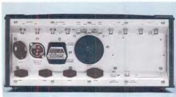
Fig 8—Rear view of 520 PAL Vectorscope. The mounting angle of the coax connectors permit connecting cables to leave the instrument without protruding excessively and with a minimum of clearance space required.
