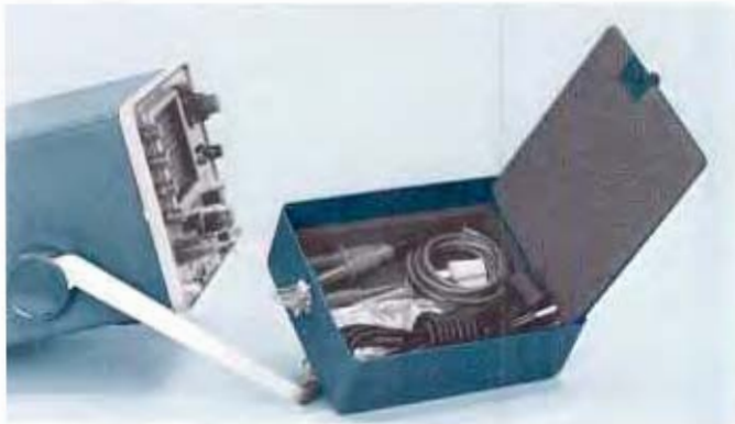
Panel cover provides storage for standard accessories.
