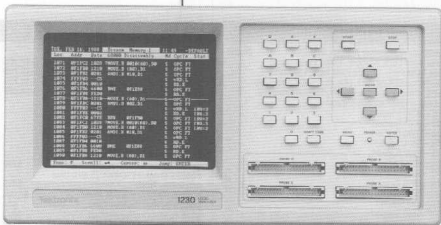
2K-deep memory can be displayed in State, Timing, or Disassembly formats. This 68000 disassembly display shows all bus cycles. Another disassembly display is also available that shows only instruction cycles and looks like an assembly listing.
