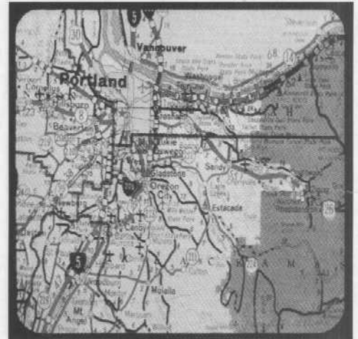
A High resolution color display permits very high information density. The map above is displayed on a 6" x 6" taut mask CRT.
