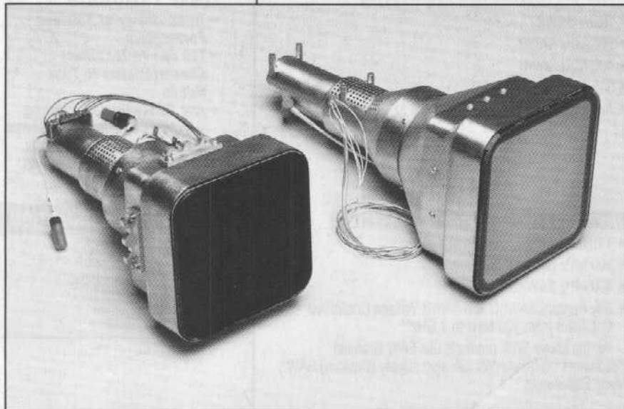
Five and six inch color avionic CRT assemblies. The CRT on left is shown with night vision compatible contrast enhancement filter.
